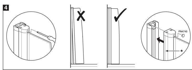
Adjust the curtain screen by tightening or loosening the top screw so that the bottom of the glass runs evenly along the bath rim. The curtain screen **MUST NOT** come out of the wall channel beyond the marked line (\*). Push fit the screw cap.
