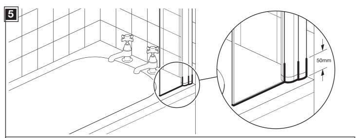
Apply silicone sealant to the outside of the curtain screen where shown.
