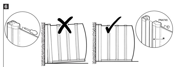
Adjust the screen by tightening or loosening the screws (top and bottom) so that the bottom seal gently brushes the bath rim evenly along its length. IF THE SEAL IS TOO TIGHT ON THE BATH THE SCREEN MAY LEAK. The screen **MUST NOT** come out of the wall channel beyond the marked line (\*). Push fit both screw caps in their **TOP** and BOTTOM positions.
