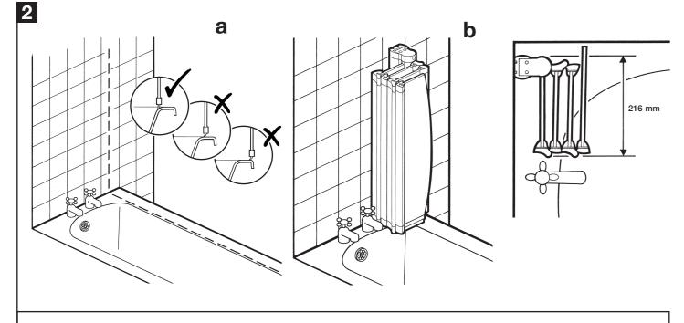
Position the screen so that it rests along the inner edge of the bath (a). It is advisable that the screen is fitted so that it will fold into the bath (b) Check the measurement above (4 and 5 panel version) to ensure you have sufficient space
