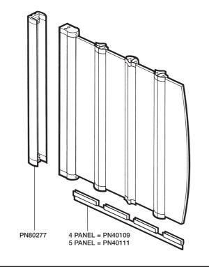
Drill three holes in the wall channel at points shown using a 4.5mm drill bit, through the grooved centre line.
