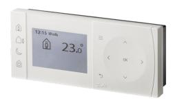
**TPOne** Programmable Room Thermostat platform delivers new levels of user friendly interaction. The flexible dot matrix display uses easy read icons and text information to provide feedback on status and settings to the installer and user. When the display is activated the backlight illuminates and guides are given on the what buttons will adjust temperatures or navigate the setting menus.
