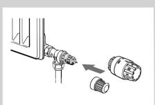
Repeat step 3 and 4 until all valves have been set correctly. Sensor may now be fitted or the valve cap temporarily refitted.
