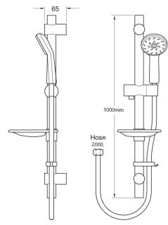
CONSTRUCTION: Stainless steel/ABS SUPPLY: Suitable For All Plumbing Systems INLET CONNECTIONS: ½" BSP WORKING PRESSURES: 0.1 - 5.0 bar CARTRIDGE/VALVE TYPE:
