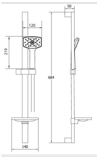
**CONSTRUCTION**: Stainless steel/ABS **SUPPLY**: Suitable For Low Pressure Systems
