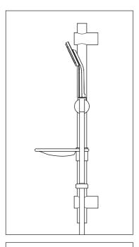
Select location for kit, ensuring no wiring or pipework in the wall can be damaged, also that when the slider bracket is positioned at the top of the rail, the hose is not over extended.
