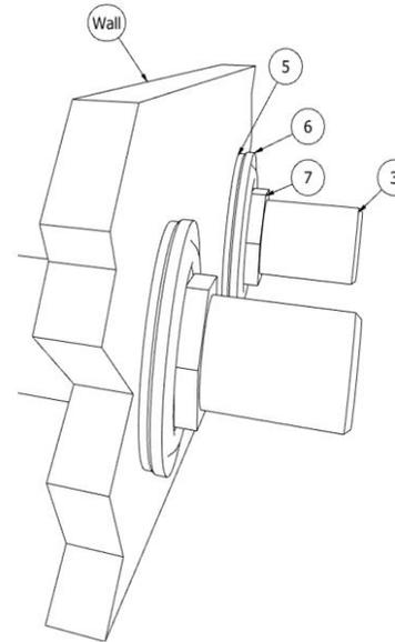
Looking at the wall from the front, the wall shrouds (4) may be screwed over the protruding unions (3) and fixed tight up to the wall.
