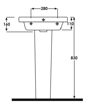
Dimensions: All measurements are in millimeters and are subject to normal manufacturing variations.
