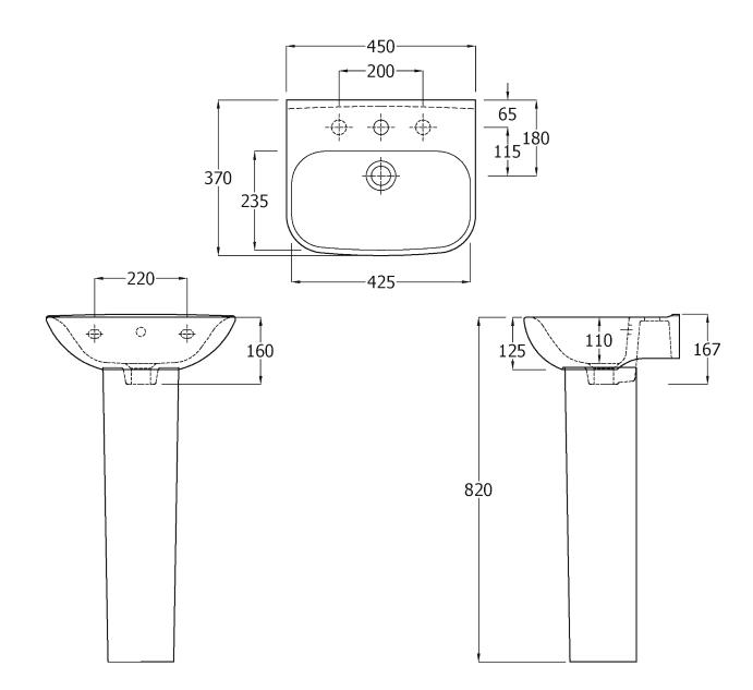
Dimensions Tolerances - Less than 75 mm.  $\pm$  5% - Not Less than 75 mm.  $\pm$  2%
