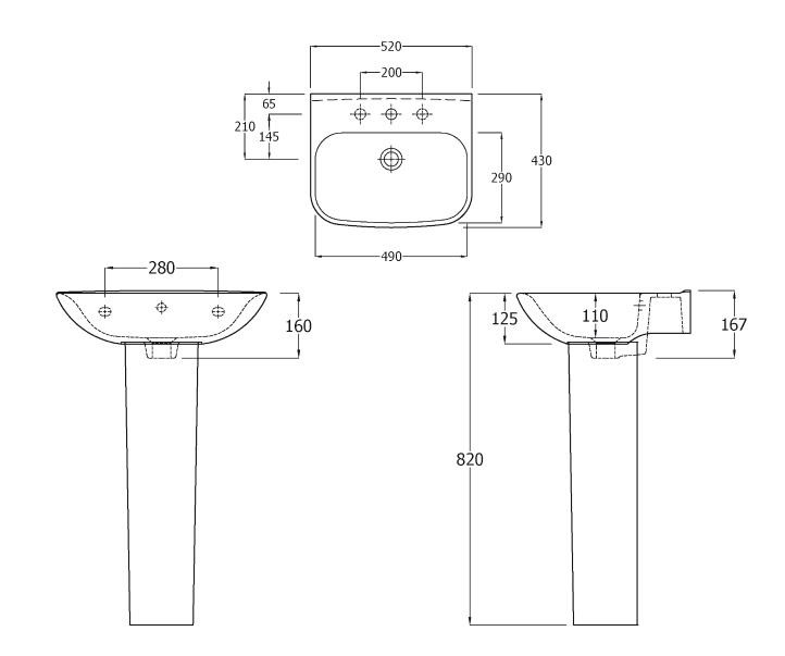
Dimensions Tolerances - Less than 75 mm.  $\pm$  5% - Not Less than 75 mm.  $\pm$  2%
