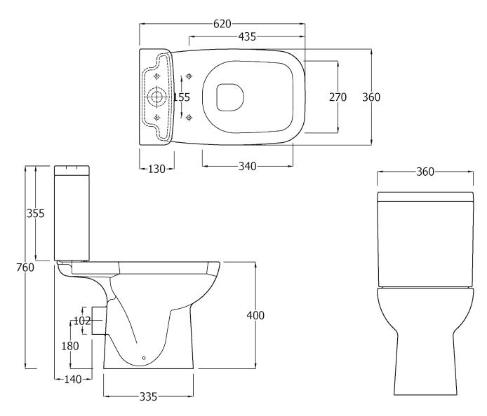
Dimensions Tolerances - Less than 75 mm. ± 5% - Not Less than 75 mm. ± 2%
