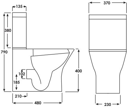
Dimensions: All measurements are in millimeters and are subject to normal manufacturing variations.
