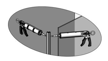
TO FIX THE OPTIONAL GLASS PANEL INTO PLACE, FIRSTLY RUN A SMALL BEAD OF SILICONE DOWN THE INSIDE OF EACH GLASS SLOT ON THE CORNER PROFILE (ITEM 15) STOPPING 5mm SHORT AT EITHER END.
