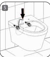
5. When you put the Pan on the threaded bars make sure that the fixings don't move and remain secure.
