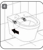
4. Then place the Pan onto the threaded bars and push it until flush to the wall, taking care of the connections which must be perfectly engaged to each other.
