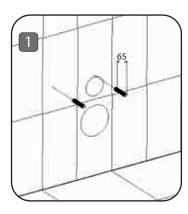
1. Prepare the waste and the fixing rods as shown in the picture and cut if necessary
