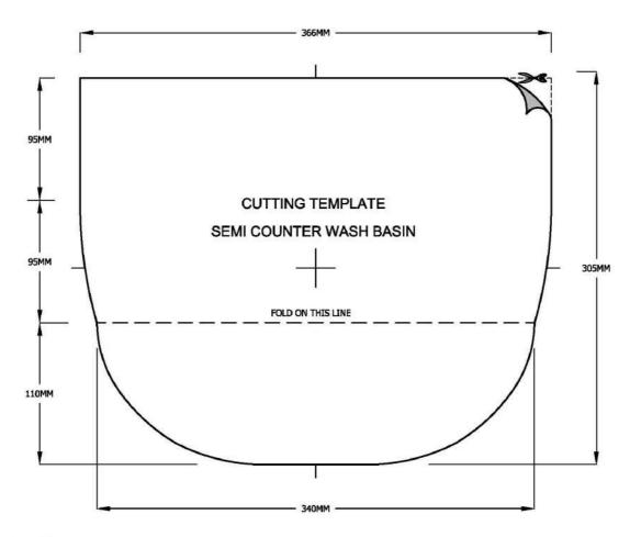
The Ceramic basins are subject to dimensional tolerances. We strongly recommend that, you use the cut out template dimensions as a guideline only & check all dimensions prior to cutting out any work tops by checking dimensions of product to be fitted.
