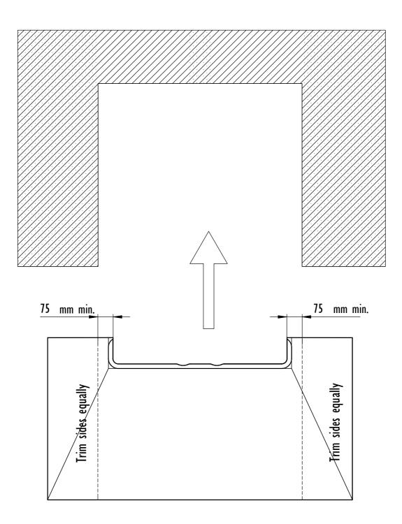
The Dec can be trimmed to fit into an alcove. (Excludes 1200x900) Ensure the Dec is trimmed equally on both sides and no closer than 75mm from the drain edge. Note: The Dec must only be cut to fit a wall to wall alcove installation, as shown. (All sizes excluding 1200 x 900)
