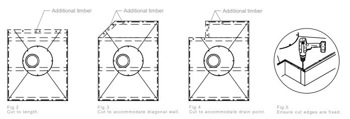
Ensure all the cut edges are supported, then drill, countersink and screw the Dec to the joists below in around 200mm intervals (avoiding pipes, electric wires, etc.). Important: Do not cut the edges that adjoin surrounding floor. Cutting the Dec may reduce flow rate performance.
