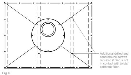
If Dec is not in contact with joist/concrete floor you must drill out and countersink the Dec to ensure it does. Failure to do this will allow unacceptable movement and may cause floor tiles to crack or become loose.
