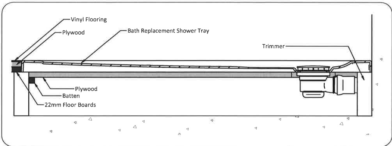
Diagram 1. Cross section of Bath Replacement Shower Tray and joists.
