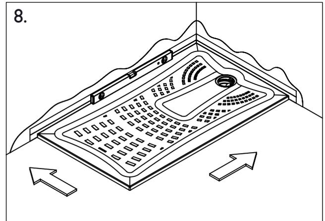
Put the tray in position and press the upstand into tile adhesive ensuring there are no air gaps. Ensure the tray is level on all four sides. Allow 24 hours before exposing to water.
