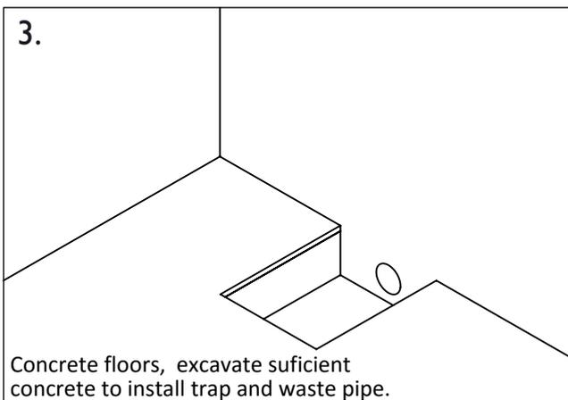
3. Concrete floors, excavate sufficient concrete to install trap and waste pipe.
