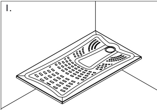
1. Determine which corner the tray is to be fitted into. This will establish which edges the fabric up stand will be attached to.
