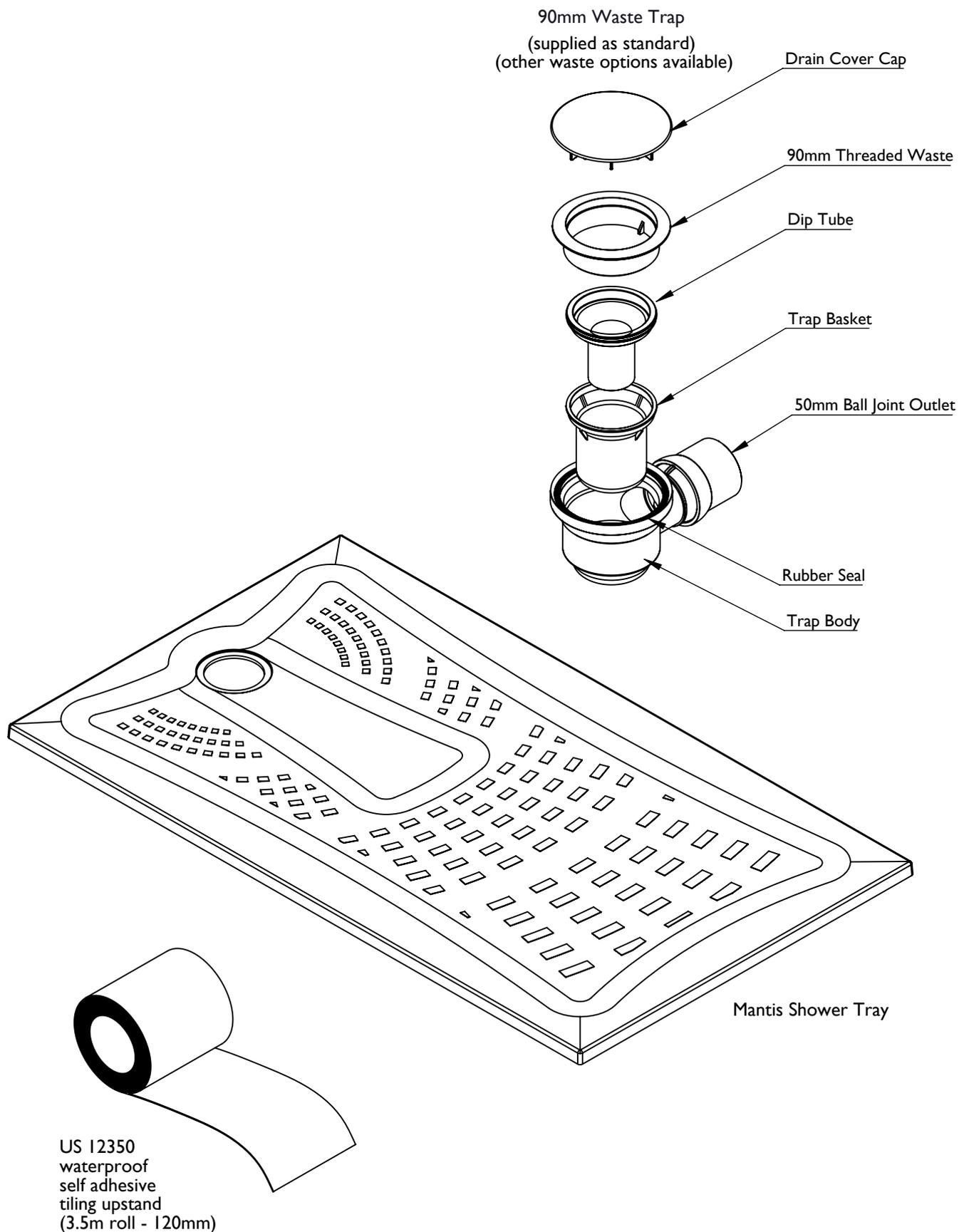
This guide is non specific to timber or concrete floors, it may refer to timber floors but in general the process of installation is the same regardless of floor type. In both cases great care must be taken when either lifting floor board or excavating the floor for waste installation.
