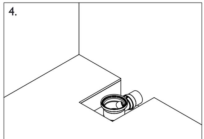
4. Position the trap so that it aligns with the hole in the shower tray and connect it to the waste pipe. Remove internal parts of the trap and place to one side, as they will be required later.
