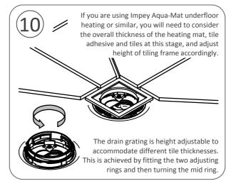
Ensure the top edge of the grating matches the finished height of your tiles -including adhesive, then glue the rings in place with ABS suitable solvent cement.
