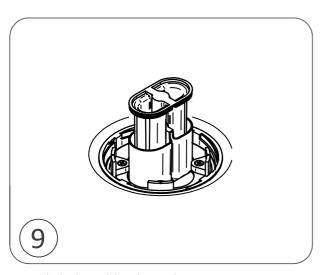
Insert the bucket and dip tube into the waste trap. Ensure they are pushed securely into position.
