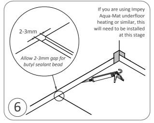
Using an applicator gun, apply sealant at all wall to wall and wall to floor interfaces, pipe entries, etc. Allow the sealant to cure before applying tile adhesive.
