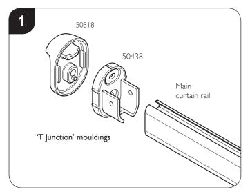
Assemble the 'T Junction' mouldings (50518 & 50438) and fit onto the end of the main curtain rail.
