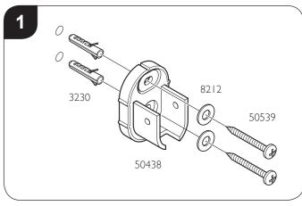
Ensuring the wall bracket (50438) is vertical, mark the hole positions and drill the wall using a 6.5mm masonry drill. Insert the wall plugs and fix the first bracket to the wall using screws (50539) and washers (8212). Repeat with the other wall bracket as required, ensuring the rail is level.
