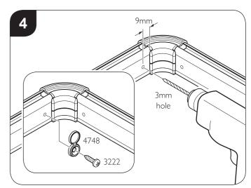
From inside the rail, drill 2x 3mm holes 9mm from the edges of the corner moulding as shown. Fix the corner moulding to the rails using 2x screws (3222) and Cover caps (4748). Repeat with any other corners as required.
