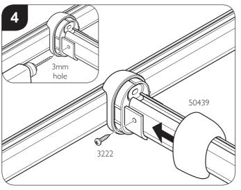
Position the rail onto the 'T Junction' mouldings, drill a 3mm through the side of the mouldings. Fix using screw (3222) and side cover (50439) over mouldings.
