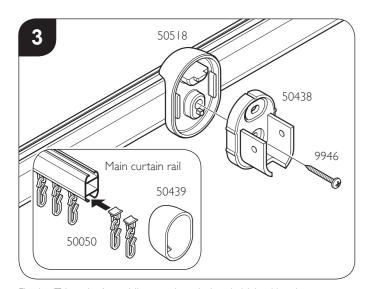
Fix the 'T Junction' mouldings to the window bridging kit using screw (9946). Assemble the hooks and gliders (50050) and slide into the bottom recess of the main curtain rail. Slide the curtain wall mount covers (50439) onto both ends of the main curtain rail.
