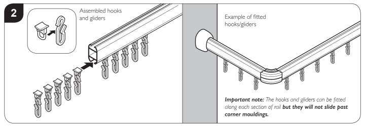
Assemble the hooks and gliders and slide into the bottom recess of the rail. Note: Insert the hooks and gliders to suit rail installation.
