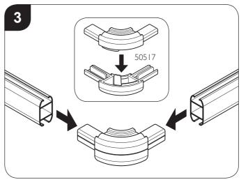
Assemble the 2x Corner mouldings (50517). Fully slide the rails onto the assembled Corner mouldings.
