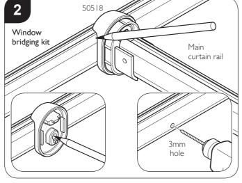
Position assembled 'T Junction' mouldings and rail against the window bridging kit in the required position. Mark around the moulding. Remove 'T Junction' assembly. Use moulding (505 | 8) as a template to mark the fixing hole. Drill a 3mm hole where marked.
