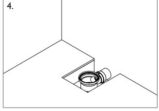
Position the trap so that it aligns with the hole in the shower tray and connect it to the waste pipe. Remove internal parts of the trap and place to one side, as they will be required later.
