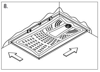
Put the tray in position and press the upstand into tile adhesive ensuring there are no air gaps. Ensure the tray is level on all four sides. Allow 24 hours before exposing to water.
