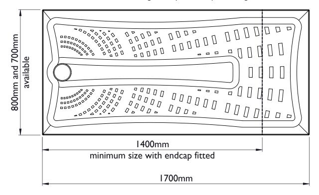
When measuring and cutting the tray please allow for the the end cap See illustration below.
