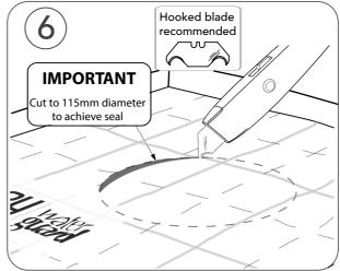
With the WaterGuard membrane lying on top of the drain and over the cutter guide, use a hooked blade to cut around the inside wall of the cutter guide. Ensure the cut is concentric with drain and Ø115mm in diameter.
