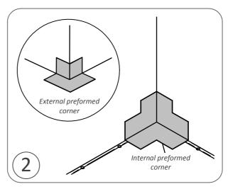
When primer is fully dry begin tanking the wetroom. Apply the internal or external preformed corner to wall to wall and wall to floor interfaces.
