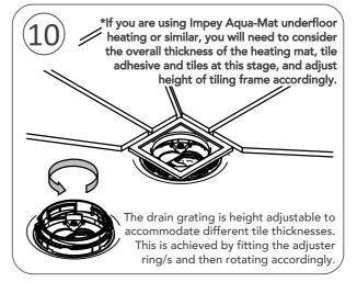
Ensure the top edge of the grating matches the finished height of your tiles -including adhesive, then glue the rings in place with ABS suitable solvent cement.
