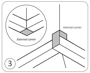
Using the 150mm jointing tape, line all the corners and wall/floor junctions so that the tape overlaps 75mm at the wall and 75mm onto the floor. Release the backing paper and smooth down by hand, ensuring the jointing tape overlaps at all junctions.
