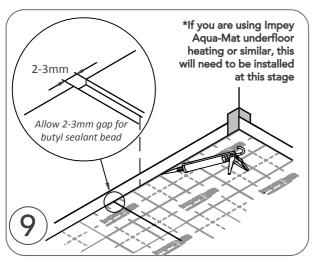
Using an applicator gun, apply sealant at all wall to wall and wall to floor interfaces, pipe entries, etc.
