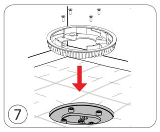
The WaterGuard clamp can now be gently pressed into place. Ensure the WaterGuard clamp is aligned with the screw bosses on the bowl and gradually ease the WaterGuard clamp into place until fully down. Then tighten the four clamp screws by hand. DO NOT USE POWER TOOLS.
