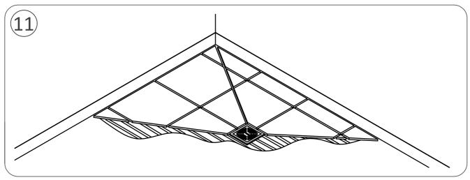
The installation of Aqua-Dec EasyFit is now finished. There is no need to apply primer to the surface of the WaterGuard. Apply tiles to the whole area. If you are using large format tiles, they must be cut diagonally to follow the falls in the Dec, e.g. from the corners of the tiling frame to the corners of the Dec. In all cases the tiles must be laid to follow the falls/gradient of the Aqua-Dec EasyFit.
