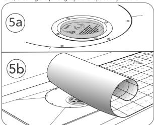
Fully locate the WaterGuard cutter guide into the bowl top (a). Measure and cut required length of WaterGuard Membrane. Remove the release paper and carefully set into position - pressing firmly onto the jointing tape (b). Ensure there are no air bubbles. Repeat steps 4 and 5 until the floor is covered.
