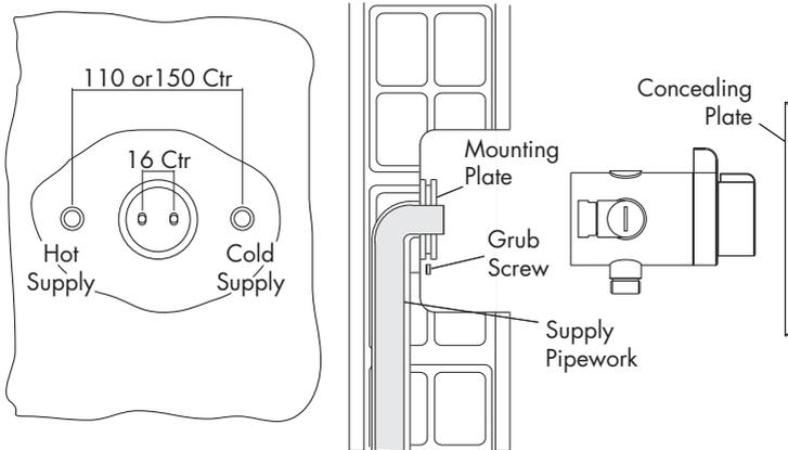
**NOTE:** Wall elbow available for concealed installation for use with flexible hose shower kit.
