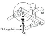
4 - Remove hot and cold inlet plugs using a 10mm Allen key
