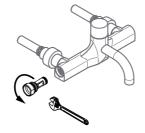
10 - Unscrew the connector plug using a suitably sized spanner and refit the check valve housing and end cover
