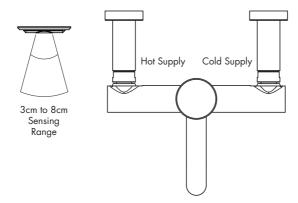
As the sensor is activated the flow of water will commence, the mixer is factory set to deliver water at a pre-set maximum temperature of 41°C.
