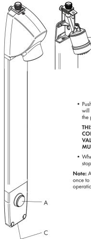
Push the operating button (A), a small quantity of water will be discharged through an outlet in the lower part of the panel (C).
