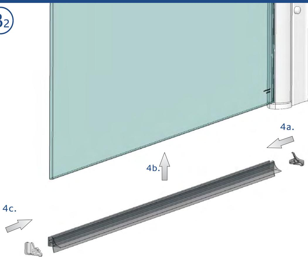
With 'drip strip' to inside, select appropriate hand seal end caps (left /right).
