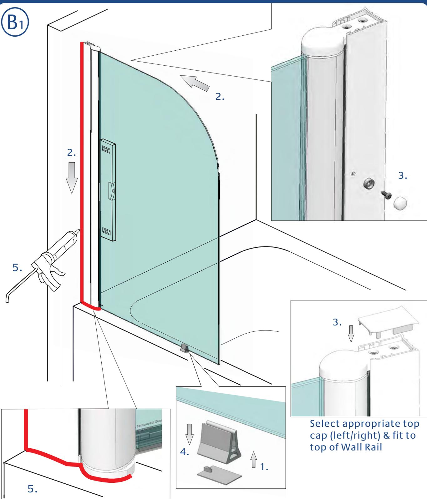
1. Push support & basepad onto bottom edge of glass toward outer end of screen.
