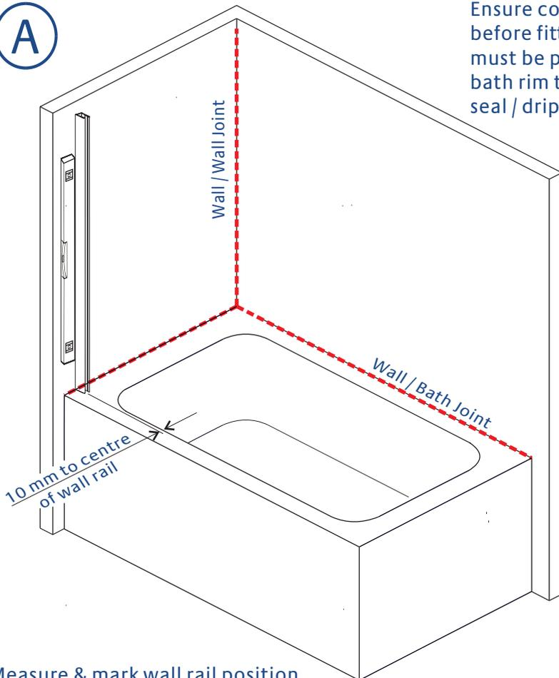
Ensure continuous silicone sealant bead as indicated before fitting wall rail. For best performance, screen must be positioned adjacent to the inner edge of the bath rim to ensure effectiveness of the bottom seal / drip strip.
