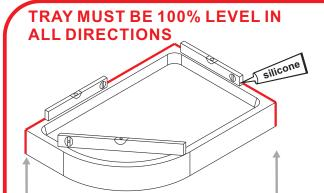
Ensure the shower tray is level in all directions and is properly sealed to the wall. The wall must be tiled down to the top edge of the tray. **Do not angle out bottom tile**.
