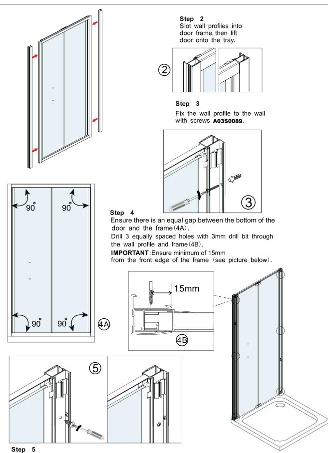
Fix the frame with screws SPOST4.
