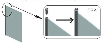
2. Unscrew one of the brackets A **BSYS021** and insert the moving panel **A**,reattached the brackets **A**. Ensure the brackets **BSYS021** are facing in the correct direction. Fig 3.
