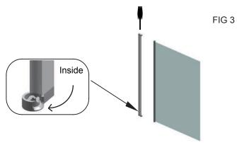
3. Position the wall profile LR8387C so the seal on the moving panel sits on the inside edge of the bath. Fig 4.
