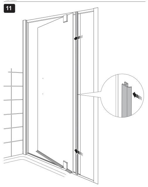
(a) Install the panel seal to the door shown above.
