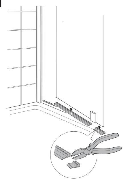
(a) Install the splash seal to the door as shown above.
