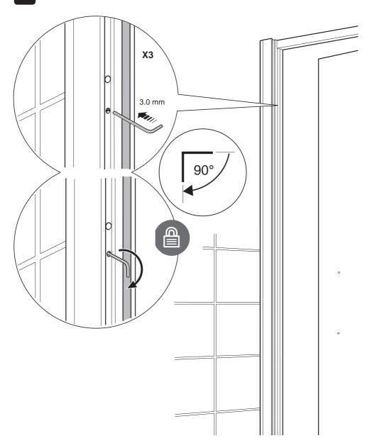
(a) Using the 3.0 mm hexagonal wrench (supplied), turn through 90° clockwise in three locations to lock the door frame in position. Repeat this on the other wall channel.
