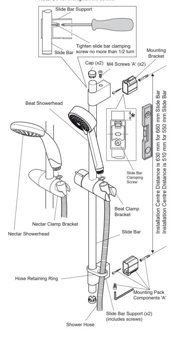
\* Note! Ensure an equal length of slide bar top and bottom.
