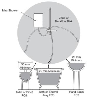
Hose retaining ring fitted and shower fittings fixed at a suitable height preventing dirty water backflow
