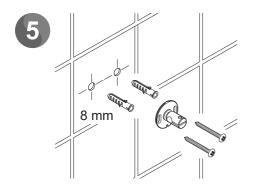
Drill the holes for the wall fixing bracket. Insert the wall plugs and fix the bracket to the wall using the screws supplied.
