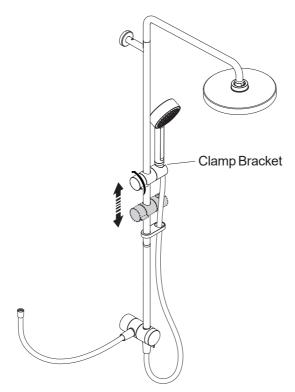
Operate the lever and slide the clamp bracket up and down until it is positioned at the desired height and lock in position.
