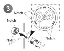
Slide the diverter partially over the wall plate ensuring the notches in the diverter lines up with the notches on the wall plate and fix temporarily in place.
