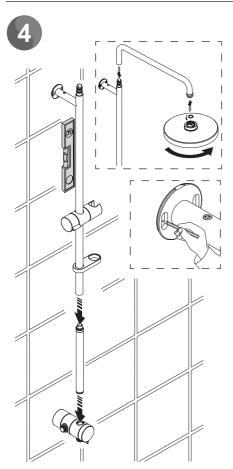
Fit the clamp bracket and hose retaining ring onto the middle bar, then screw into the lower bar. Loosely fit the wall bracket into the middle bar arm with the grubscrew hole at the top.
