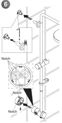
Loosely fit the concealing cover onto the middle bar. Ensure the lower bar is fitted correctly.
