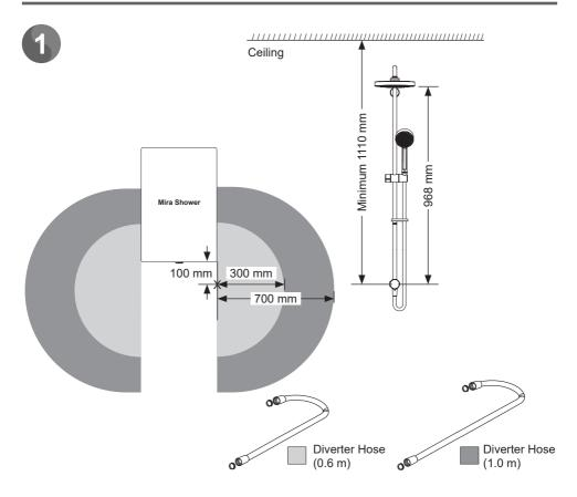
If the diverter is positioned outside of the light grey area as shown in the diagram a longer link hose is available up to 1.0 m max in length.
