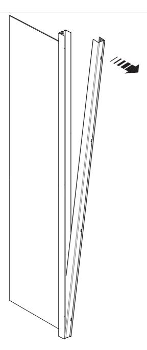
(a) Remove the wall channel from the panel.
