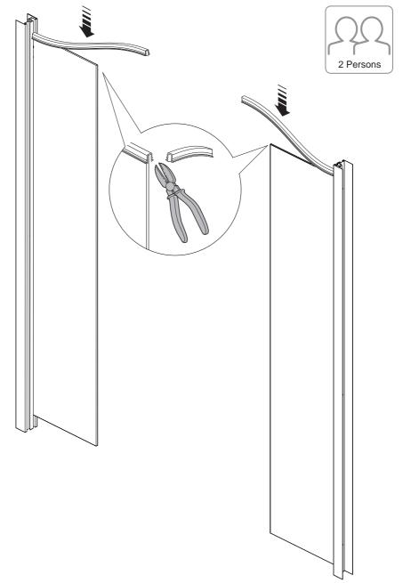
(a) Install the seals to the top of the panels as shown above and cut to length, leaving 5 mm extra to allow for shrinkage.
