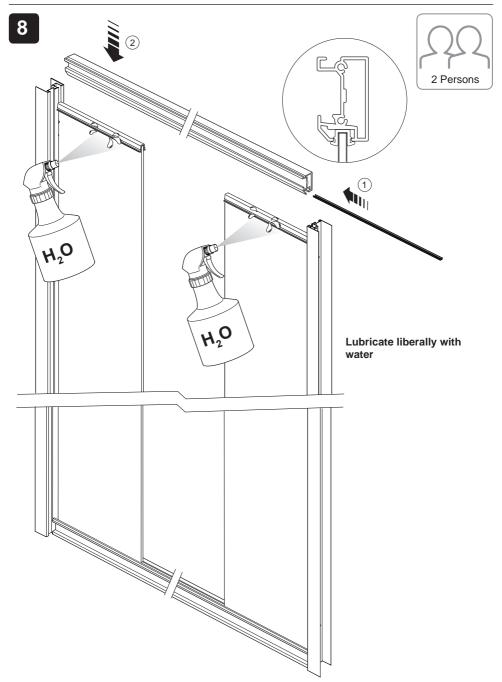
(a) Slide the track infil into the middle of the channel and lower the track onto the seal.
