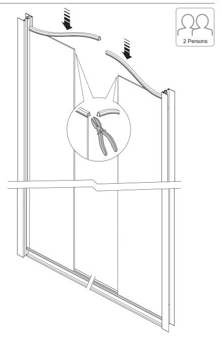
(a) Install the seals to the top of the panels as shown above and cut to length, leaving 5 mm extra to allow for shrinkage.
