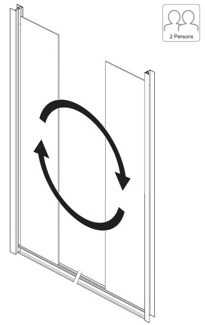
(a) Carefully turn the whole assembly through 180 degrees.
