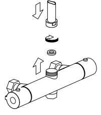
Install the riser into the top outlet of the shower valve.
