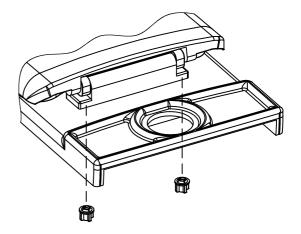
LOCATE THE SEAT BOLTS INTO THE SEAT MOUNTING HOLES AND USE THE NUTS TO FIX THE SEAT IN PLACE ON THE UNDERSIDE.
