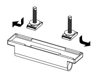
SLIDE THE BOLT ASSEMBLIES INTO THE SLOTS ON THE UNDERSIDE OF THE SEAT BARREL
