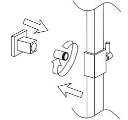
Fit the wall bracket to the riser kit
