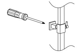
Make sure the riser is level, mark the position of the screw holes on the wall bracket. 6
