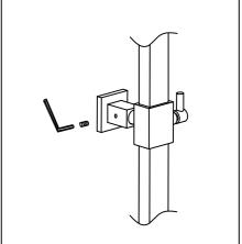
Install the riser on the wall bracket, tighten the screw.
