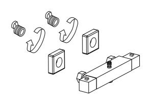
Fit decorative covers over the offset connectors. Then insert sealing washer into nut and tighten onto offset connectors with wrench, being careful not to damage the chrome finish on the connecting nuts.
