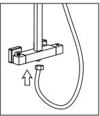
Connect the shower hose to the bottom outlet on the shower valve, and screw the conical end to the shower handset. Place the conical end of the shower flex into the parking bracket on the riser rail.
