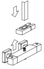
Install the riser into the top outlet of the shower valve.
