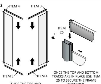
SLIDE THE TOP AND BOTTOM TRACKS; LH & RH, INTO THE GLASS PROFILES UNTIL FLUSH.
