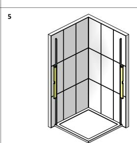
MAKE SURE THE WALL PROFILES ARE TRUE WITH A SPIRIT LEVEL. MARK THROUGH THE FIXING HOLES WITH A PENCIL. REMOVE PROFILES, DRILL AND PLUG THE WALL, (ITEM 27). THE WALL PLUGS SUPPLIED MAY NOT BE SUITABLE FOR YOUR SUBSTRATE, USE SUITABLE FIXINGS. NOW REFIT WALL PROFILES IN PLACE USING ITEM 22, 23 & 24.
