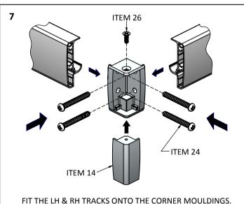
ENSURE THAT THE TRACKS ARE SQUARE AND TRUE BEFORE SECURING THE CORNER MOULDINGS TO THE TRACK WITH ITEM 24. ALSO FIT THE CORNER MOULDING CAPS; ITEM 14, WITH ITEM 26 REPEAT FOR BOTTOM TRACK.
