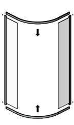
SLIDE THE TOP & **BOTTOM TRACKS** INTO THE GLASS **PROFILES UNTIL** FLUSH.
