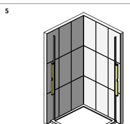
MAKE SURE THE WALL PROFILES ARE TRUE WITH A SPIRIT LEVEL. MARK THROUGH THE FIXING HOLES WITH A PENCIL. REMOVE PROFILES, DRILL AND PLUG THE WALLS (ITEMS 22). THE WALL PLUGS SUPPLIED MAY NOT BE SUITABLE FOR YOUR SUBSTRATE, USE SUITABLE FIXINGS. FIX THE WALL PROFILES IN PLACE USING ITEM 20.
