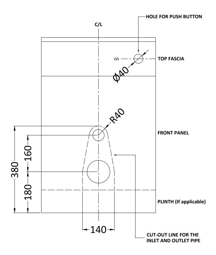
MARK OUT THE OPENING ON THE FRONT PANEL FOR THE INLET AND OUTLETS OF THE W.C. PAN. FOLLOWING THE ABOVE DIMENSIONS, CHECK THE SIZE AGAINST THE PAN BEFORE CUTTING OUT. DO NOT CUT OUT THE BOTTOM PLINTH!
