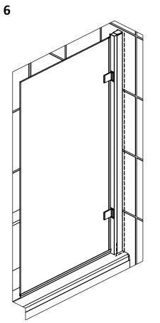
EXTERNALLY SILICONE SEAL THE WALL PROFILE WHERE IT MEETS THE WALL AND 150mm HIGH AS SHOWN IN THE DEATILED VIEW BELOW. ALL IN A CONTINUOUS BEAD.
