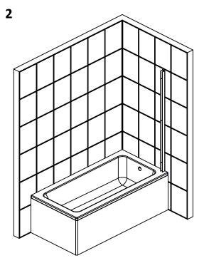
DRILL AND PLUG THE WALL WHERE YOU MARKED FOR THE FIXING HOLES. THEN FIX THE WALL PROFILE IN PLACE USING THE LARGE FIXING SCREWS OR SUITABLE FIXINGS.
