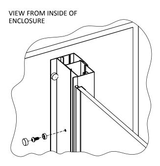
TO PIN YOUR SCREEN IN PLACE USE THE 3mm DRILL BIT TO DRILL THROUGH THE HOLES IN THE WALL PROFILE.
