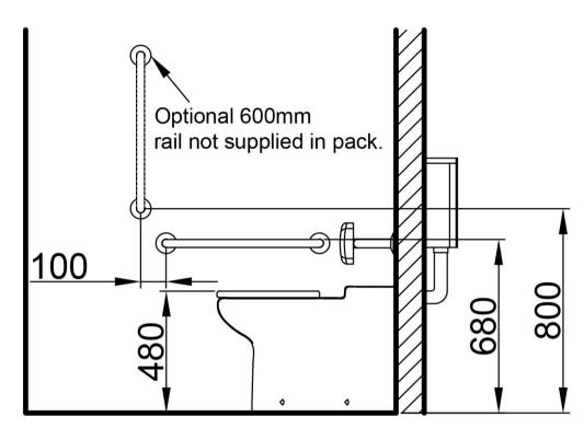
Above is for guidance only, refer to relevant building regulations (Only Nymas components shown. See data sheet for pack components).
