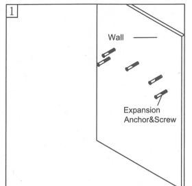
Fix the position of mounting holes on wall depend on the actual dimension of Stainless Steel Brackets(a total of 5holes)
