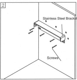
Lock the screws on the wall in turn
