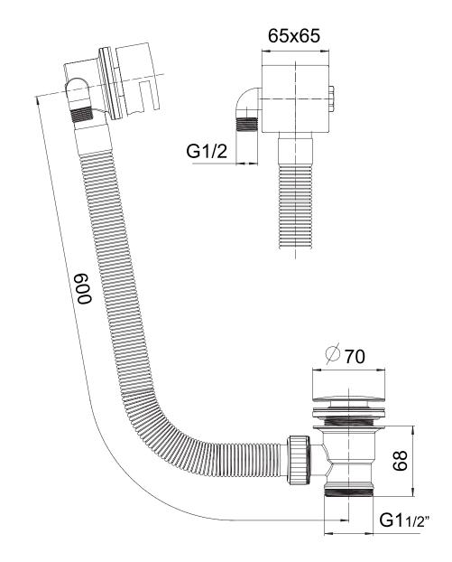
Dimensions (measurements in mm)
