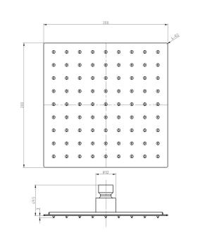
Dimensions (measurements in mm)
