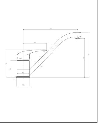
Dimensions (measurements in mm)
