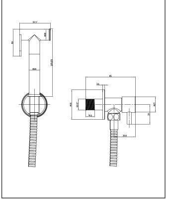
Dimensions (measurements in mm)
