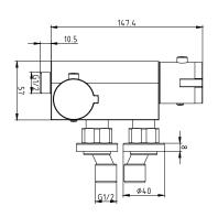
Dimensions (Measurements in mm)
